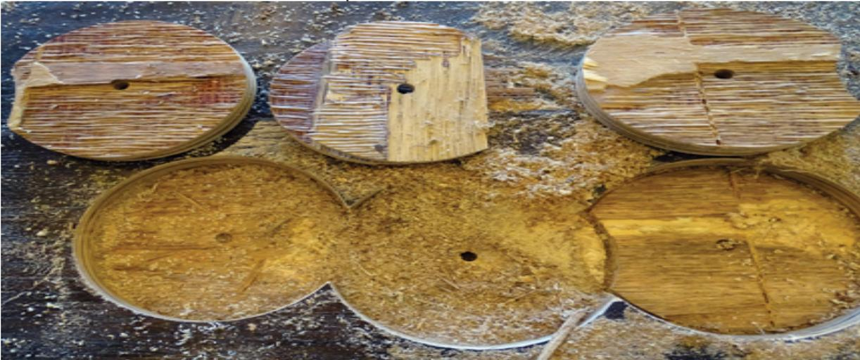
Wood fibers can clearly be seen attached to the adjoining layers of these pucks cut with a hole saw. The failure was caused by wood shear, not delamination.
